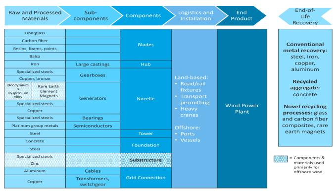
Figure 1. Land-based and offshore wind supply chain overview
