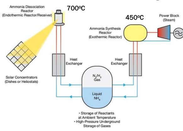
The projected installed cost of ammonia based CSP with six hours of storage  $13/kWh_{th}$  (less than SunShot target of  $15/kWh_{th}$
