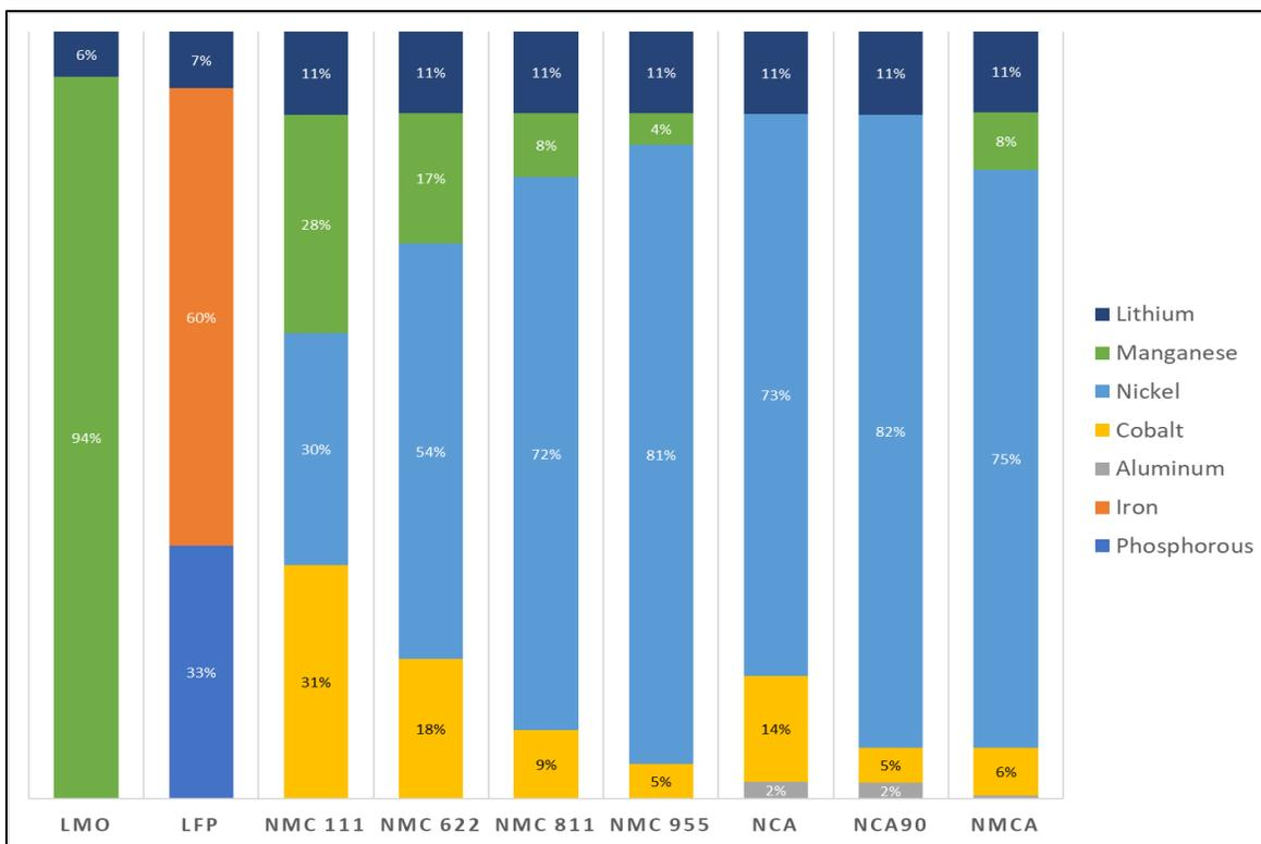
Figure 1. Metal content (wt%) of lithium-ion battery cathodes.
