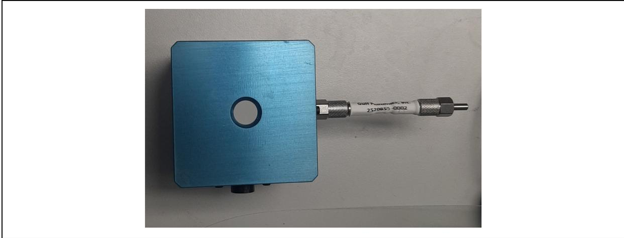
**Figure 3-4: Small integrating sphere used in initial measurements.**
