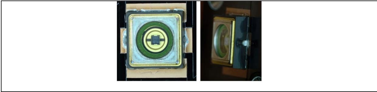
Figure A-13: Front-view and oblique view of UV-5 LED.
