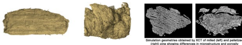
Simulation geometries obtained by XCT of milled (left) and pelletized (right) pine showing differences in microstructure and porosity
