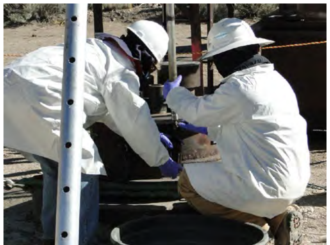
Technicians collect samples from a groundwater well at the NNSS.
