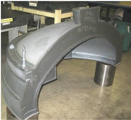
Lower Reactor Head
