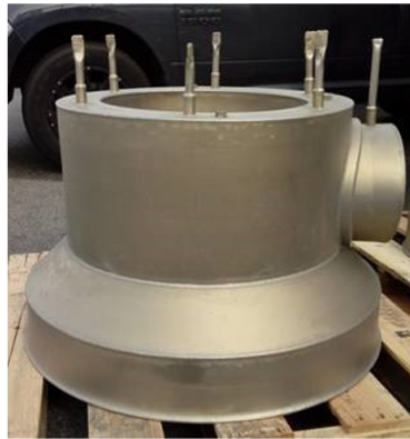
Steam Plenum Access Port
