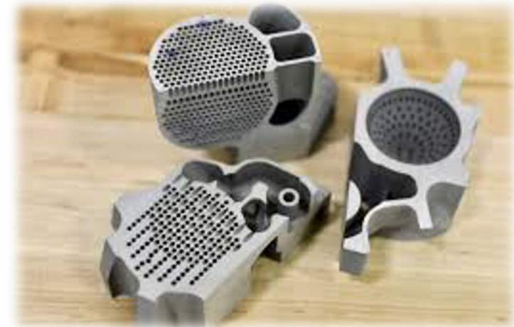
AM-produced heat exchanger (GE)
