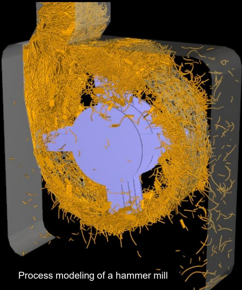
Process modeling of a hammer mill
