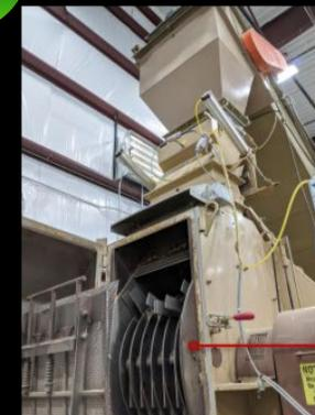
Material jamming in hammer mill grinder
