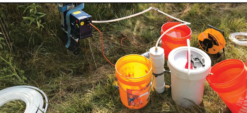
During this redevelopment of a well using a surge block, the purged water was filtered through activated carbon.
