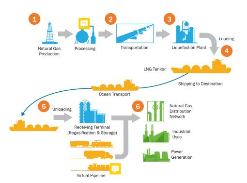
degrees Fahrenheit (-162 degrees Celsius), **reducing its volume by 600 times. LNG is a clear, colorless, and non-toxic liquid,** which is stored in large cryogenic tanks until it's loaded into an LNG tanker.
