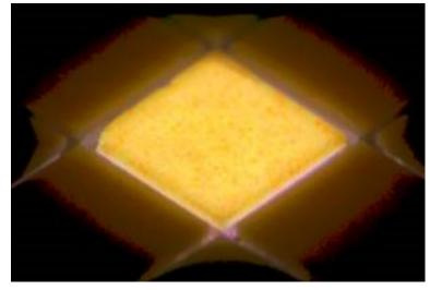
Lumileds' prototype high-luminance LEDs in dense array, with center LED lit up.
