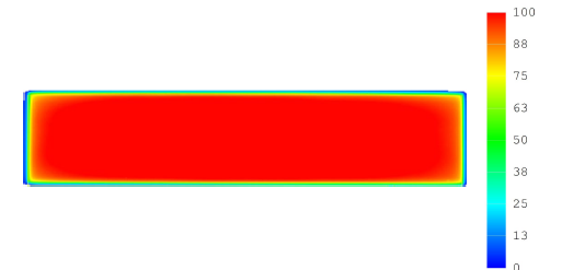
Figure 22: Typical luminance distribution for a Brite 3 Rectangle Level 1. Operation conditions: vertical in air, RT (= 25 °C), I = I_{\text{max}}
