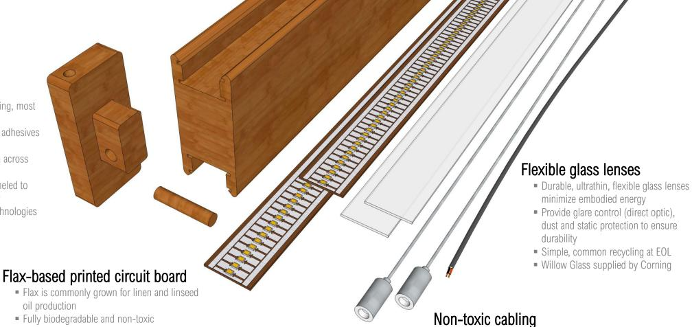
Small gauge low-voltage DC wire minimizes
