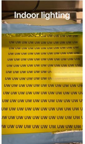
Edge-lit device from the glass waveguide
