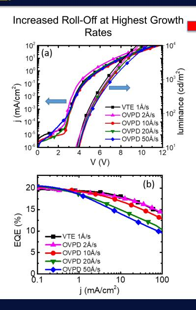
Heterogeneous Nucleation of Defects at High OVPD Growth Rates
