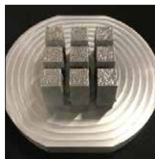
Figure 9. Molybdenum bulk test build.
