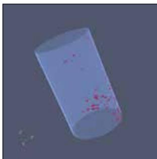
Figure 5. 3D digital twin (red dots indicate pore detection).
