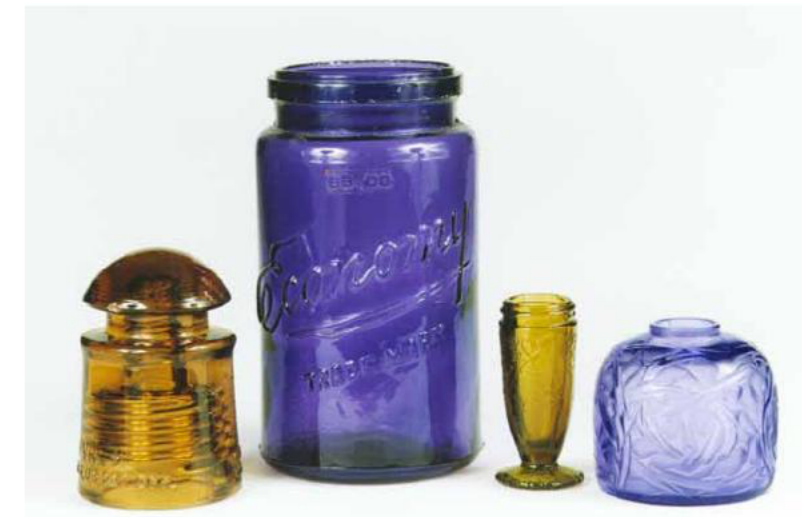
Irradiation can change color of glass
