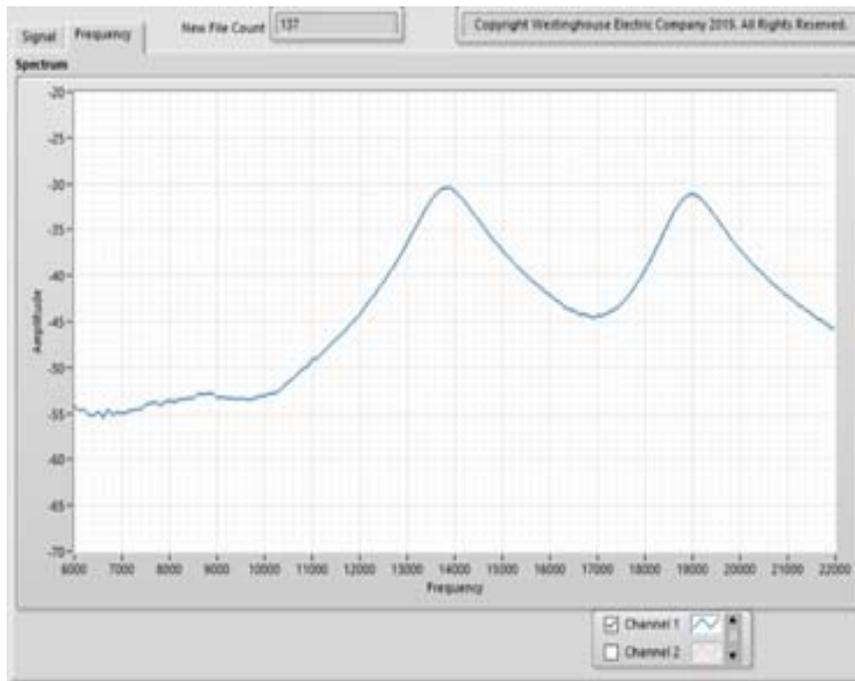
*Two sensor signals resolved in frequency domain*
