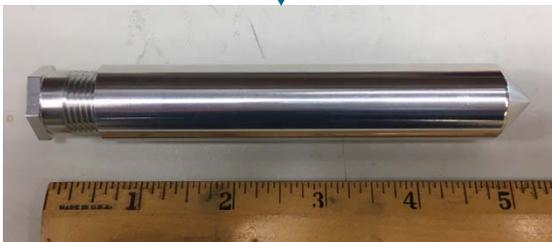
New AM transmitter with vacuum pulled inside enclosure
