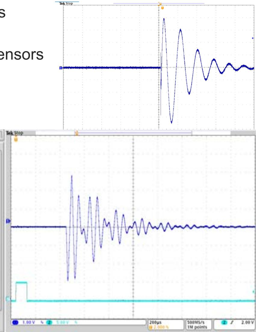
*Two sensor signals mixed in the time domain*
