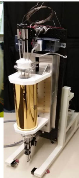
LVDT Calibration Test Rig
