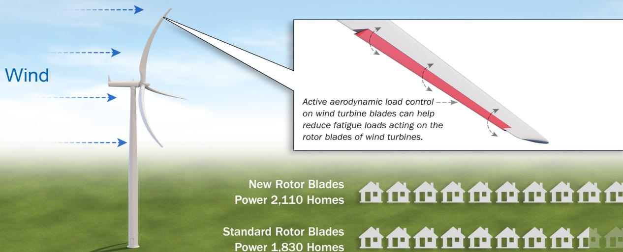
Larger wind turbine rotors can increase capacity factors, or the amount of power a turbine outputs on average over the course of a year. Assuming two turbines of the same height—one standard wind turbine with a capacity factor of 0.45 versus another high-energy-capture machine with downwind, highly-flexible blades and a capacity factor of .5175 (a 15% increase)—the high-energy-capture machine can power roughly 280 more homes. *Illustration by Besiki Kazaishvili, NREL*
