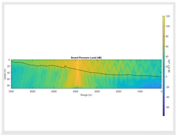
Figure 28. An example file using the Paracousti tool that shows the sound pressure level for a continuous source off a coastline.
