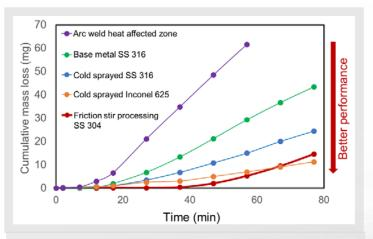
Figure 13. Friction stir processing and cold spray are both types of solidstate processing that dramatically outperform arc welding and base metal by demonstrating better cavitation erosion resistance.
