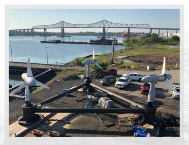
Figure 34. Verdant's Free Flow System turbines positioned on the TriFrame mount.
