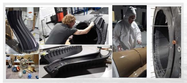
Figure 15. To link automated design to additive manufacturing, the grand prize winner of the I AM Hydro Prize, Team Cadens Hydro, completes post-print processing, fabrication, fit, and finishing steps. Their winning concept may radically reduce costs for micro/small hydro parts and tools and increase annual energy production.
