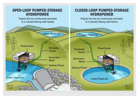
Figure 7. Generic comparison of open- and closed-loop PSH projects.
