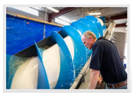
Figure 17. Percheron Power's composite Archimedes hydrodynamic screw.
