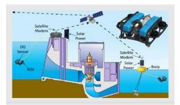
Figure 12. The autonomous water quality monitoring system increases the reliability of water quality data collection around hydropower facilities. The data are collected via a robot, to be retrieved anywhere with an internet connection.
