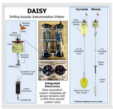
Figure 26. Schematic depicting the DAISY device instrumentation and components.
