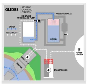
Figure 4. GLIDES during the charging phase of operations.
