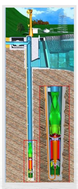
Figure 6. In Obermeyer's PSH configuration, a turbine-generator is placed at the bottom of a shaft with a lifting mechanism to facilitate future maintenance. In generation mode, water flows through the penstock into an inner pipe to run the turbine-generator and comes out through the outer pipe to the tailrace. An underground powerhouse is not required, allowing for more economical development while reducing geological risk.
