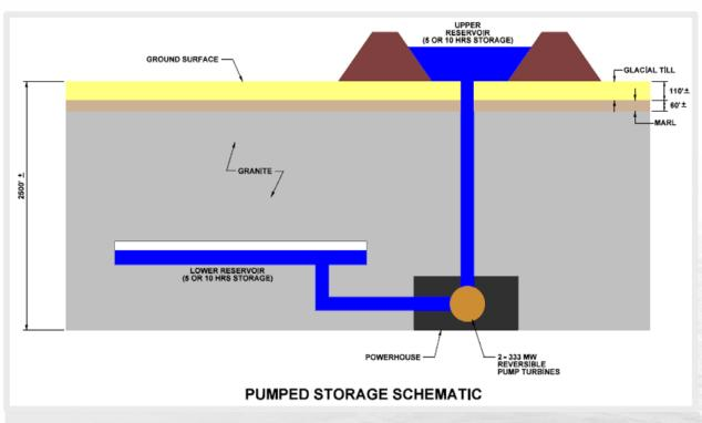
Figure 2. Conceptual closed system underground pumped hydroelectric storage concept by Nelson Energy.
