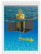
Figure 23. The University of Hawaii Hālona WEC team's proposal focused on a mobile, wave energy-powered, self-charging ocean-observing platform.
