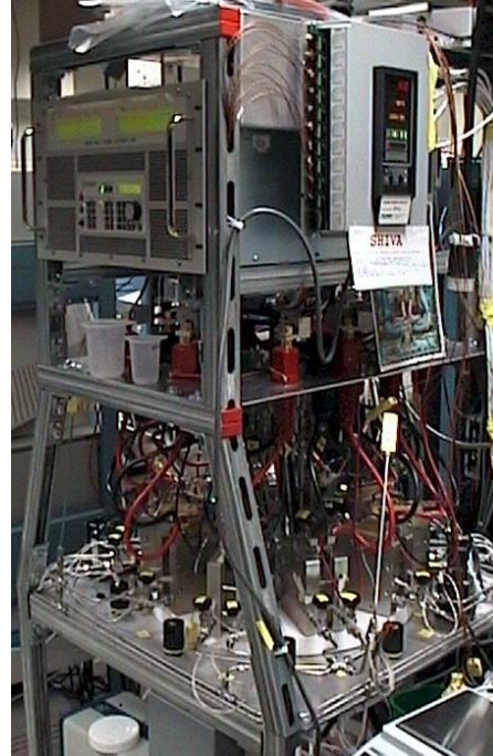
10 cell accelerated durability station (load cycle protocol)
