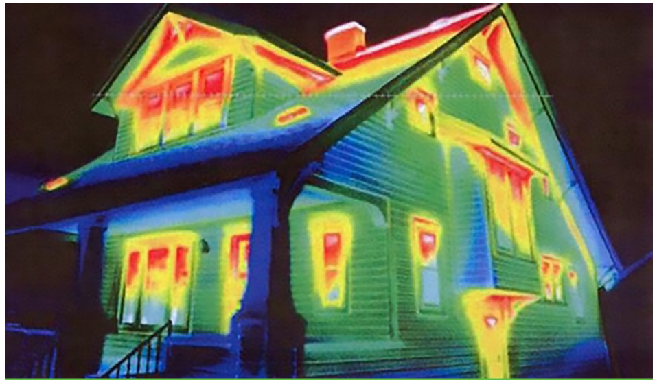
Example of windows as weak points in a home's energy efficiency.
