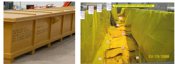
Figure 1. On the left is the exterior of B-36 disposal container. On the right is Tank 28F salt sampling drill string and lead blankets in the B-36 box.
