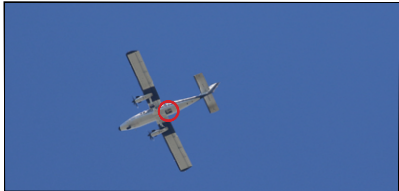
Figure 2: The National Ecological Observation Network (NEON) Airborne Observation Platform (AOP) flying over the project site. The hyperspectral camera onboard the aircraft is indicated by the red circle.
