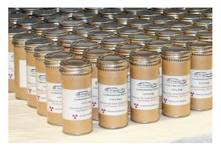
C126B – Pu Metal Standard: NBL PO, Los Alamos National Laboratory, and the Savannah River Site have begun collaborating on the production of CRM C126B Pu metal to replace C126A. The tenth in a series of Pu standards dating to 1962, this material serves as the nation's primary plutonium assay standard and is also utilized in international safeguards and nonproliferation efforts.
