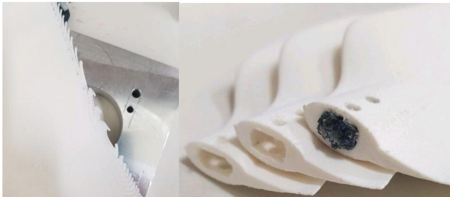
Figure 10: Blade quality from 3D Printing with ABS Material, lengthwise (L) and widthwise (R).
