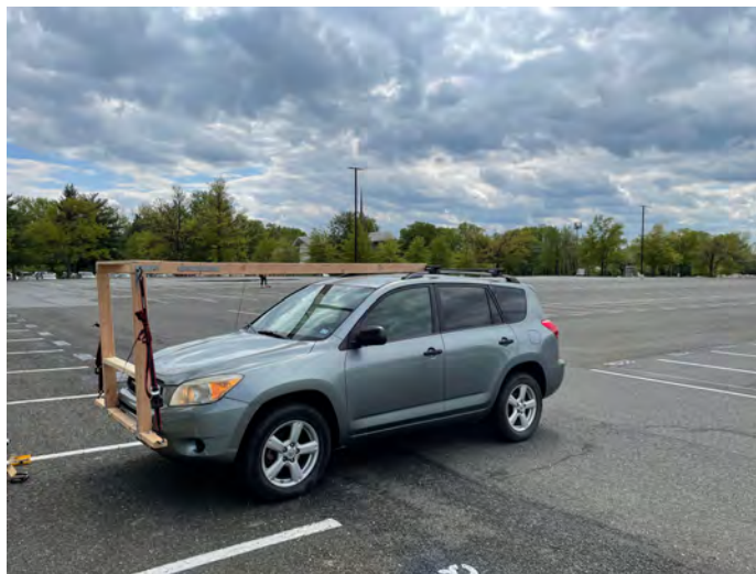
(a) Side-view of a Toyota Rav4 outfitted with the testing-rig made of 2x4's, ratchet straps, and a lot of screws
