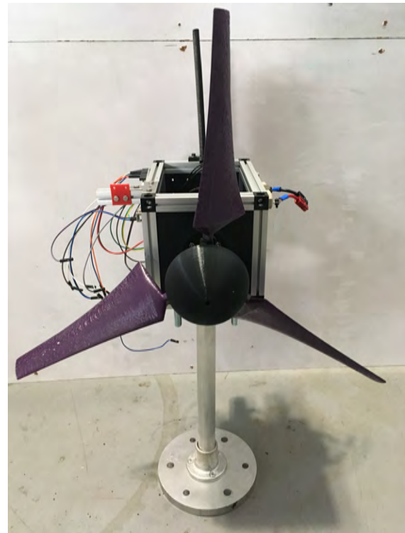
(b) Front view of unfeathered wind turbine
