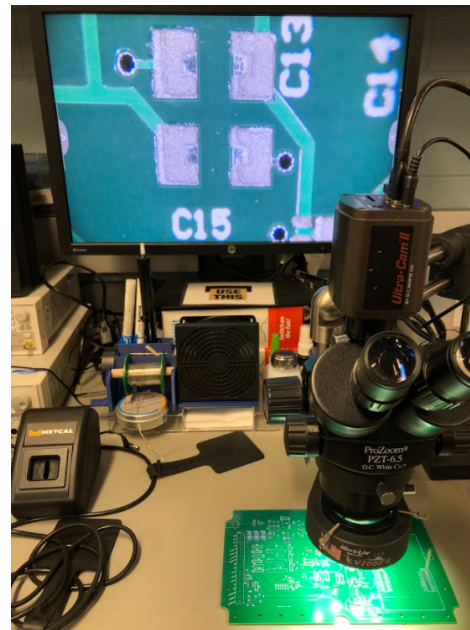
Figure 12. Electrical Assembly a) Solder paste application process. b) Microscope used to verify uniform coating of solder paste on metal pads during initial PCB assembly.
