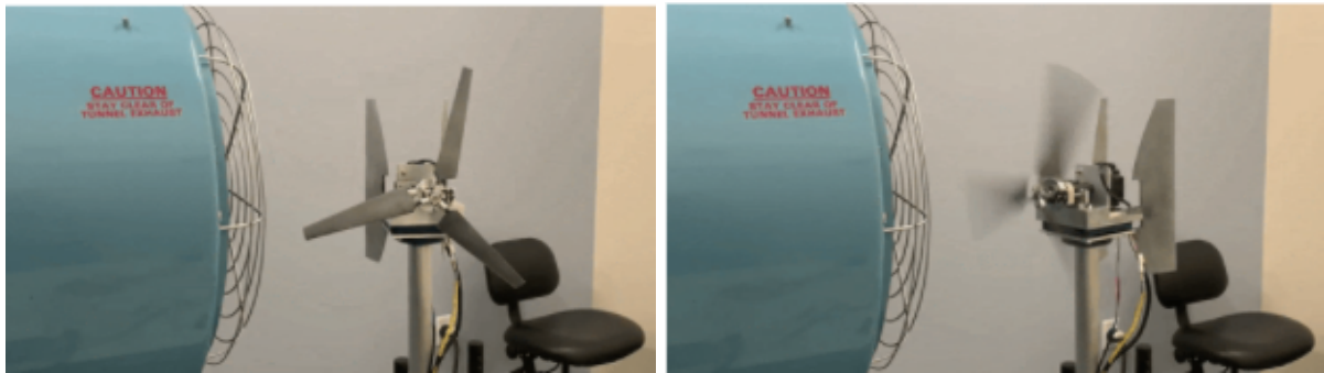
Figure 3. Demonstration of Passive Yaw System a) Turbine in yawed flow. b) Turbine after aligning with airflow and capturing energy. Note the stability of the passive yaw system when aligned with the airflow.
