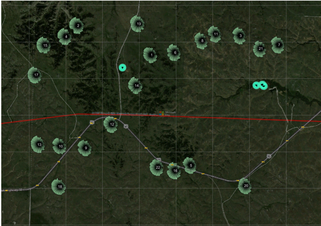
Figure 2. Rosebud Site Layout including turbines (numbered), relevant buildings (teal), 115kv transmission line (red), and existing roads including US-18.
