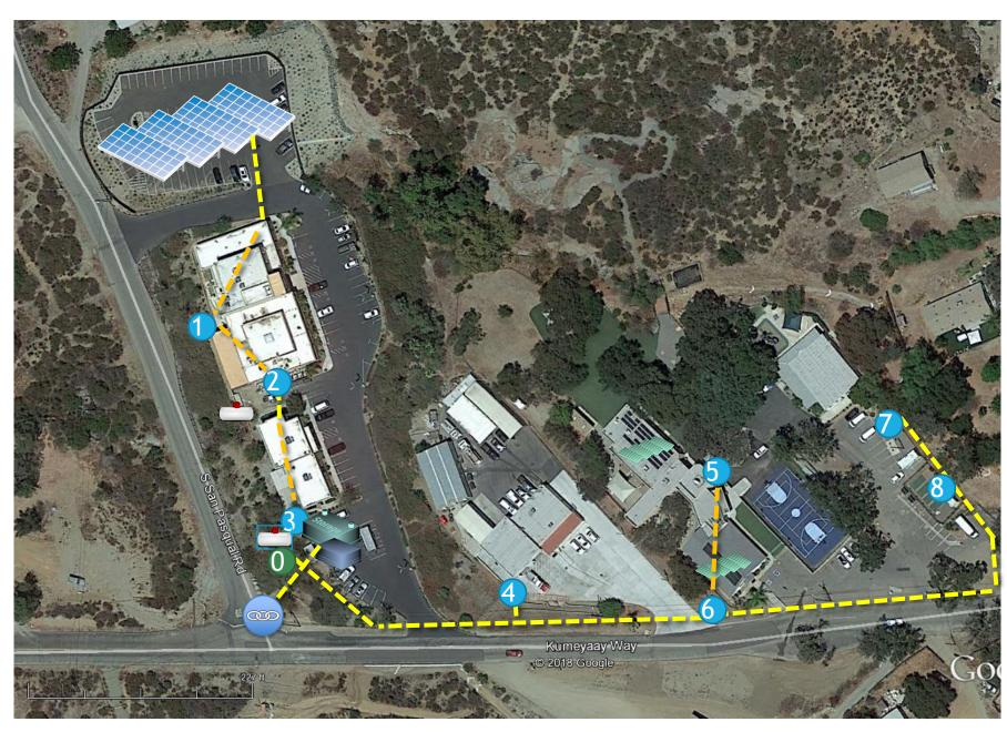
San Pasqual Tribal Government **Complex Microgrid Project CONCEPTUAL DESIGN** # Master Meter Existing/Sub Meter (# New Solar PV Site Existing Solar PV System BESS Location LP Genset Location Point of Interconnection Underground Cable Run Building Cable Run **Existing Propane Tank** New Propane Tank .
