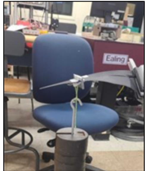
Figure 7: Blade strength testing to verify the factor of safety. The load applied was resolved to the spanwise location of the resolved lift distribution at the quarter chord. The Nylon 12 blades had high strain but did not yield.
