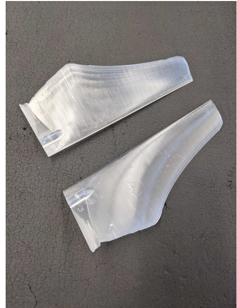
Figure 2: Accura60 material blades are stiffer than the Nylon 12 blades.
