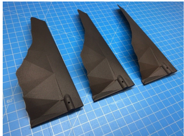
Figure 1: The Nylon 12 material blades experienced high tip deflections and were prone to flutter
