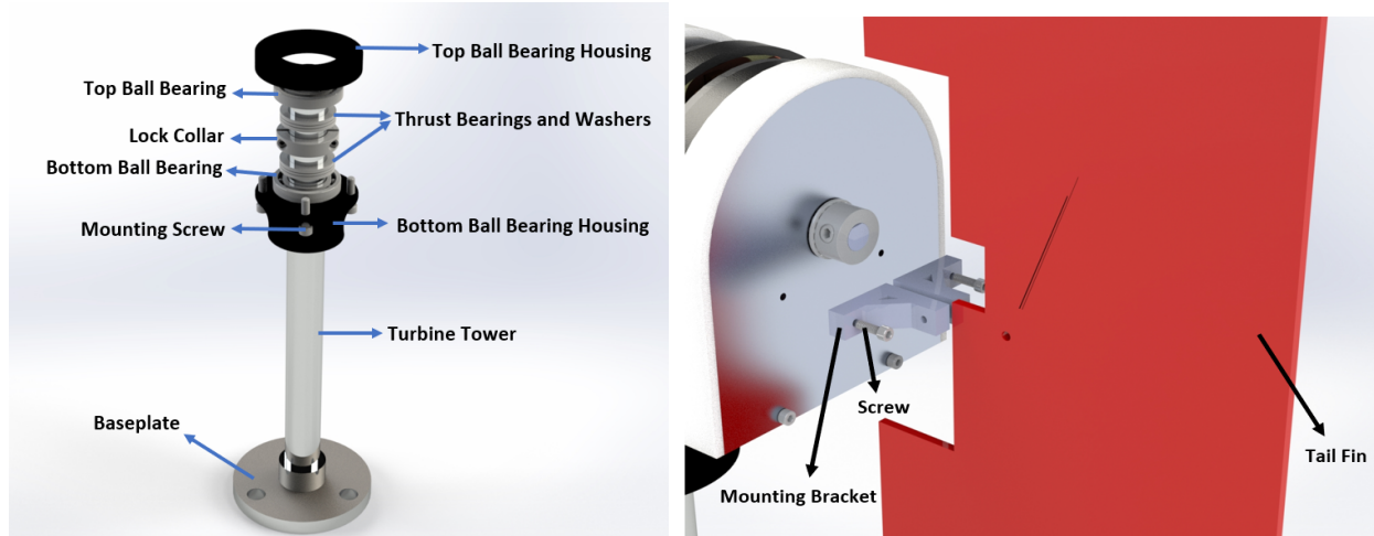
Figures 12 & 13: Exploded Views of Passive Yaw System
