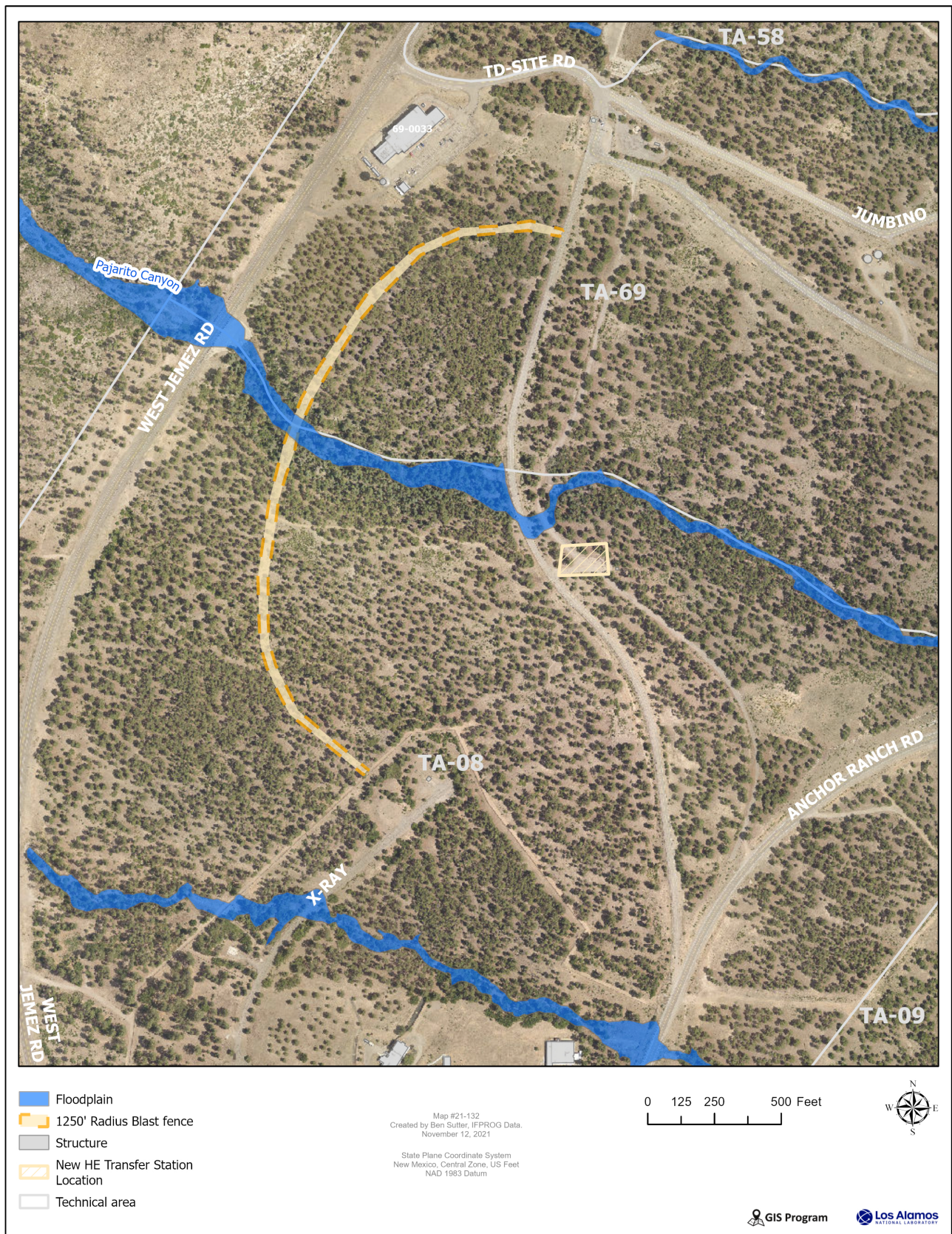
Figure 1. Map of the proposed blast radius fence line for the TA-08 HE Transfer Facility showing Pajarito Canyon 100-yr floodplain.
