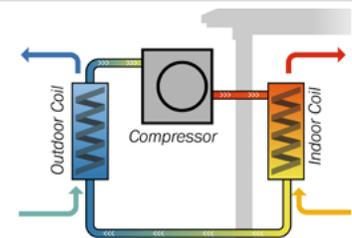
Outdoor coil absorbs heat from the air, then the compressor concentrates the heat, and finally the indoor coil releases heat into the air.
