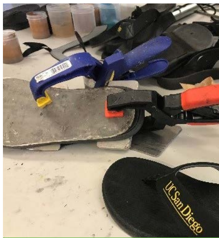
An algae-based flip-flop prototype made by Algenesis in their UCSD laboratory. Photo courtesy of Daniel Fishman, BETO
