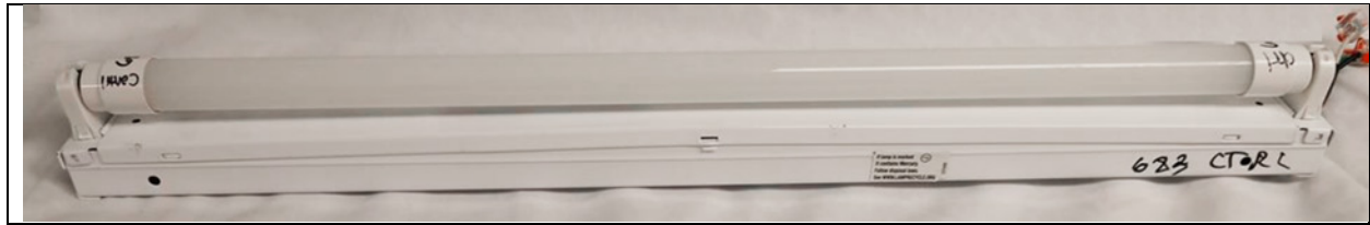
Figure A-1: Product NB-1 in a traditional fluorescent lighting fixture. The LED tube is 2 ft long.
