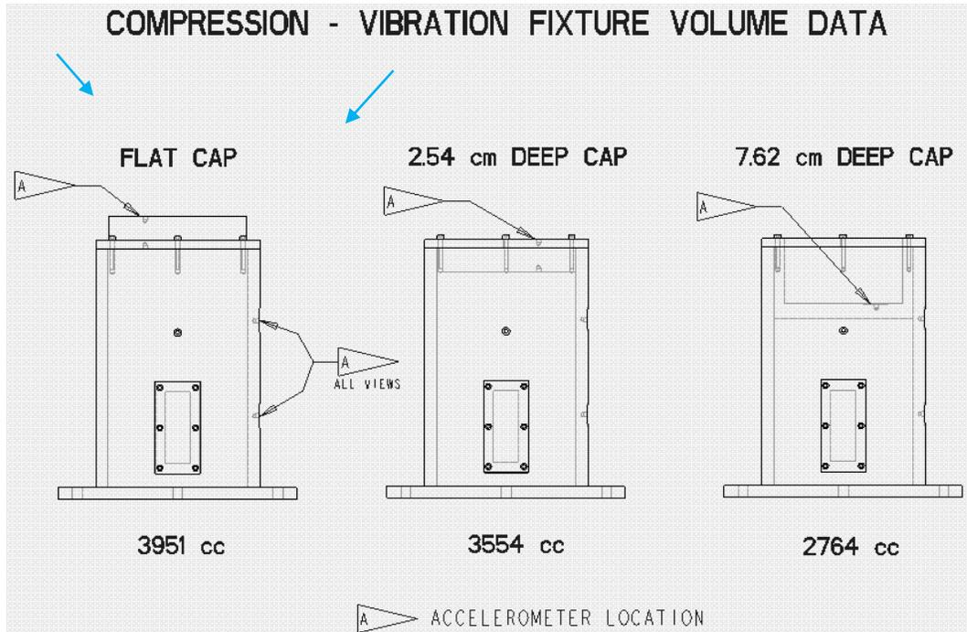
Vibration test fixture showing accelerometer locations and compression levels by different caps.
