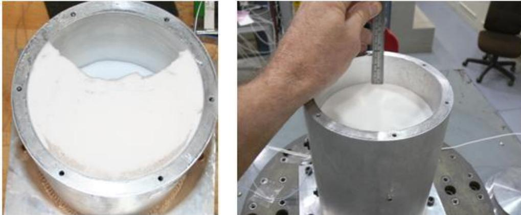
High Density Perlite exhibited compaction in the range of 13-17% after X-axis vibration (left) and Z-axis vibration (right). Photographs of typical results.
