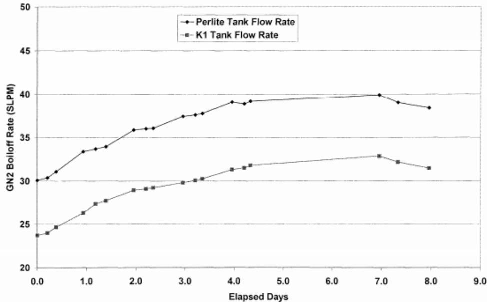
NER comparison test #1: perlite vs. K1 bubbles
