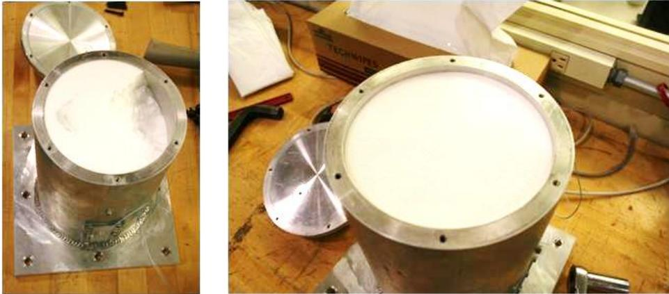
K1 Glass Bubbles after X-axis vibration, 4% void (left) and after Z-axis vibration, 2.5% void (right). Photographs of typical results.
