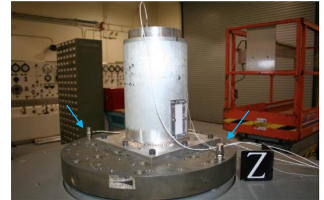
Lateral (X,Y) vibration test fixture with arrows pointing to response accelerometers (left photo) and vertical (Z) vibration test fixture with arrows pointing to control accelerometers (right).
