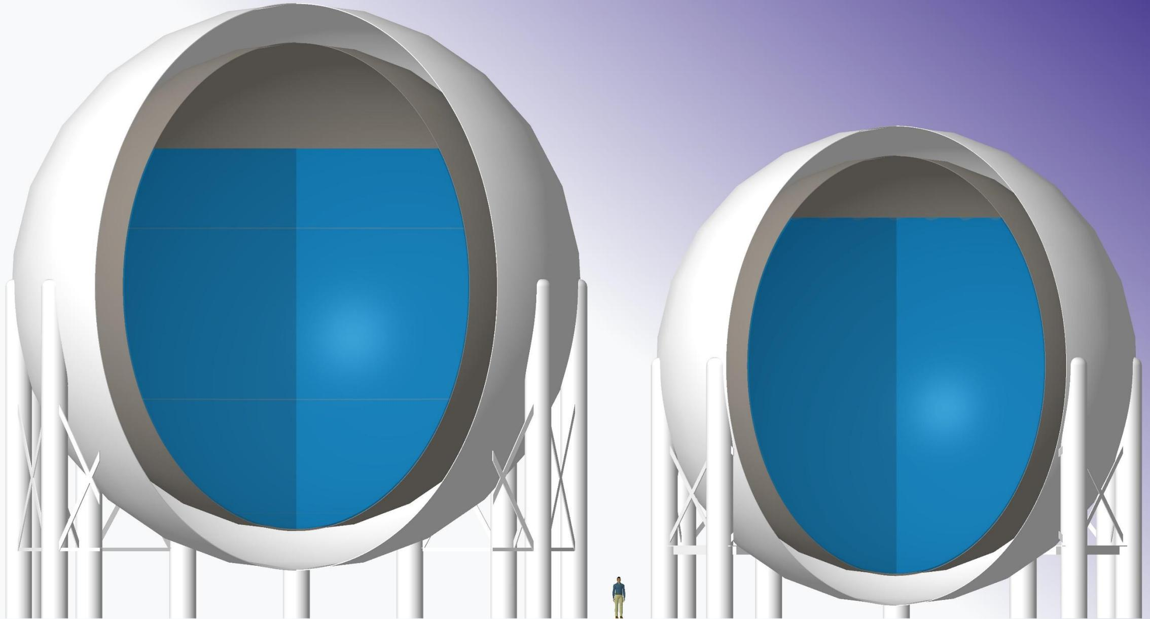
*Scale comparison of new 4,700-m<sup>3</sup> storage tank (left) and Apollo-era 3,200-m<sup>3</sup> tank (right)*
