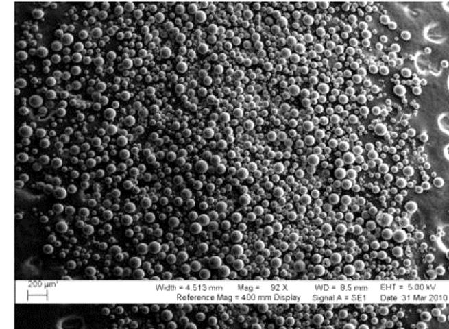
**G**lass Bubbles in the VTF before and after X / Z Random Shaker vibration: Glass Bubbles showed little degradation based on several samples. Typical micrographs 92X magnification.
