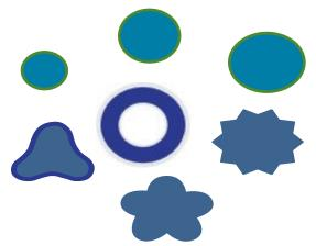
Project team is assessing various approaches to designing and producing carbon fibers with varying geometry with potential to costeffectively improve compressive performance for carbon fiber materials for the wind industry
