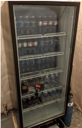
NAMA Vending machines at ORNL for leak testing
