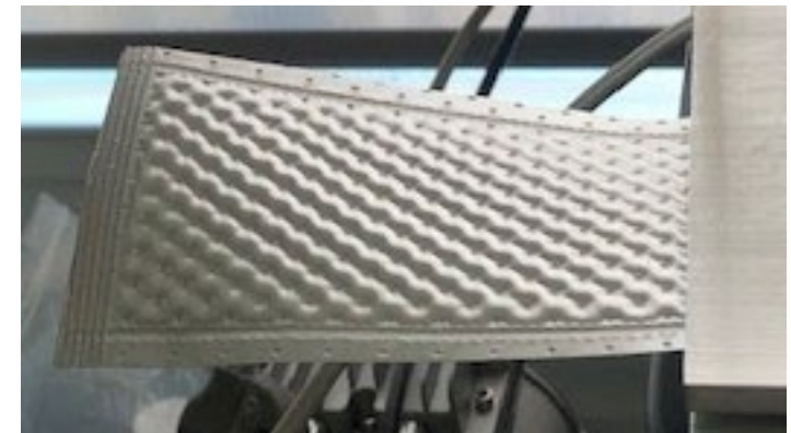
Ultrasonically welded multilayer material sample undergoing burst testing at 20 psi
