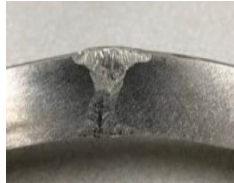
EPRI - 740H Seam Welded Pipe
