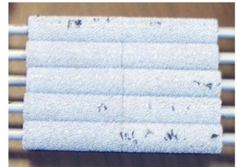
A metal foam enhanced tube bundle.
