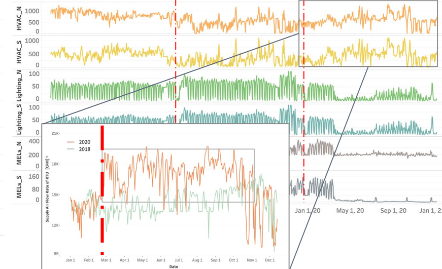
Change of HVAC operation (supply air flow rate) during the pandemic
