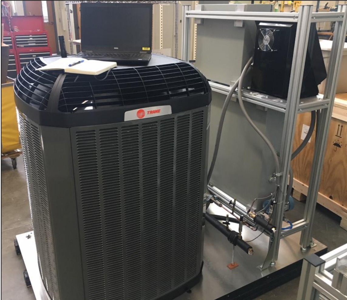
Charge subsystem – Condensing unit from Trane, modified by Emerson
