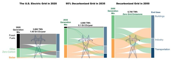
Grid mixes and energy flows in 2020, 2035, and 2050, as envisioned in the Solar Futures Study. Newly electrified loads from buildings, transportation, and industrial sectors mean that the electric grid will deliver more energy in 2035 and 2050. This energy will come almost entirely from solar and other zero-carbon sources.
