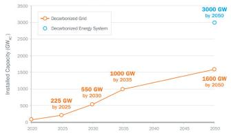
A large expansion in the amount of installed solar energy (shown here in gigawatts AC) plays a key role in decarbonization. Preliminary modeling of an additional scenario, beyond Decarb+E, in which the entire U.S. energy system is 100% decarbonized, would require about 3000 gigawatts of solar deployment.
