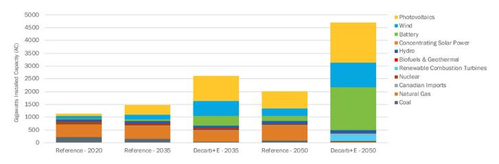
Generation capacity on the U.S. electric grid under the study's three scenarios over time. Solar, wind, energy storage, and renewably fueled combustion turbines (CTs) all play a key role in decarbonization.
