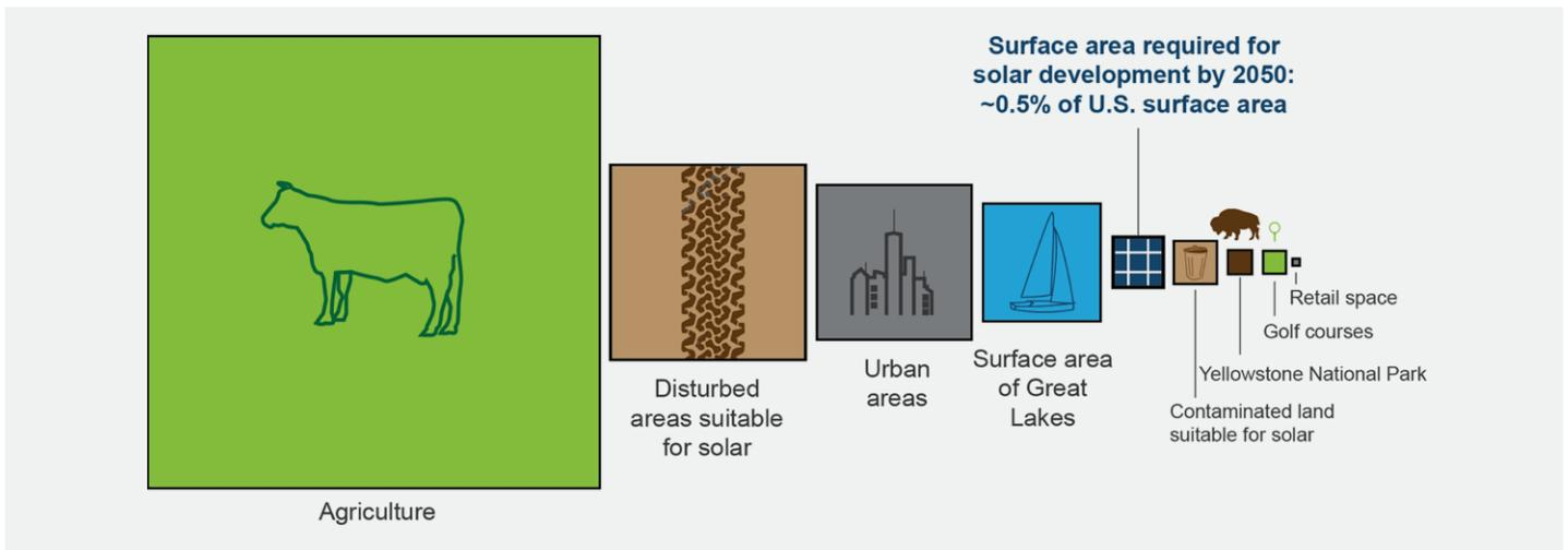
The level of solar deployment envisioned in the study would require less space than many other current land uses. This calculation does not account for siting of solar on rooftops or bodies of water, or over farm fields.
