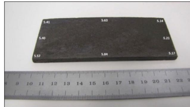
Polymer derived ceramic densified plate
