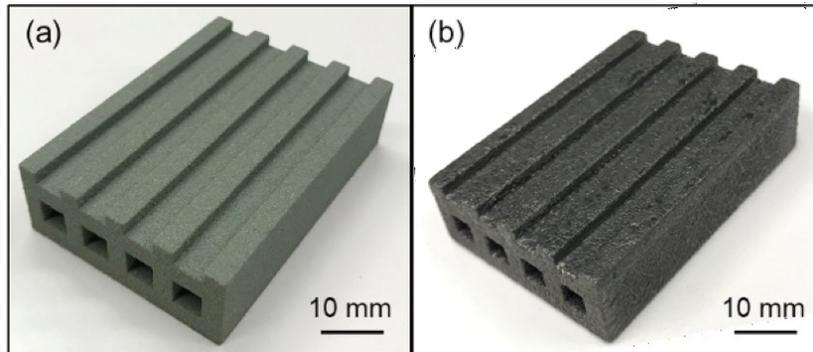
Printed green part with channels and post densification
