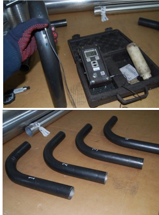
Tube Bending (courtesy of Tebunus Tube Bending/John Cockerill) – 2” Diameter Welded Tubing
