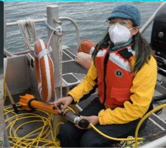
SeaSpy2, calibrated by Erin Walters, measures the generated magnetic fields
